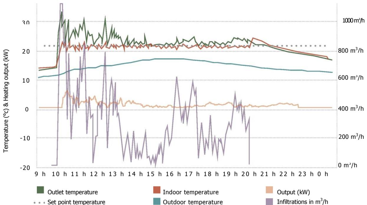
**Figure 3** Example of outdoor air infiltration of a store through the doors (in purple)
