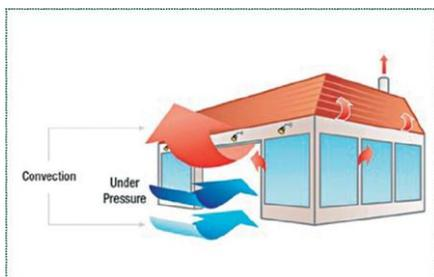
**Figure 1** Movement of air through an open door.
